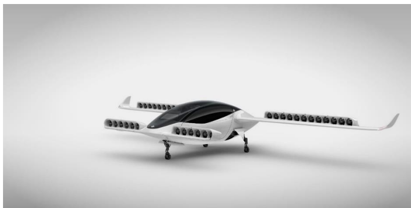
Figure 20. Lilium Jet with distributed electric propulsion
