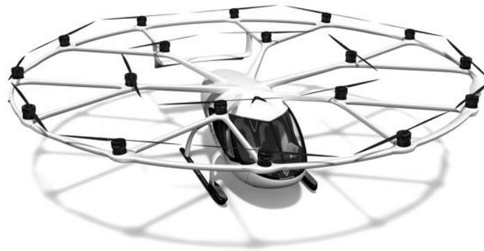
Figure 19. Volocopter – VoloCity with 18 rotors
