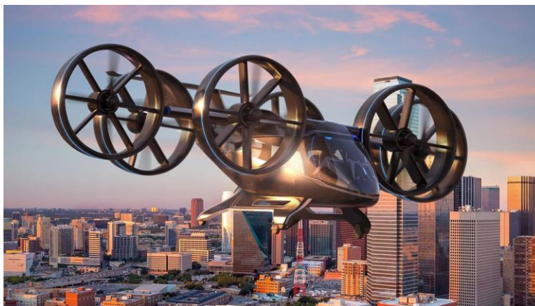
Figure 21. Bell Nexus 6HX with ducted rotors
