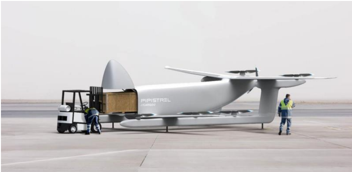
Figure 9: Pipistrel Nuuva V300 ibrid-electric cargo drone [28]
