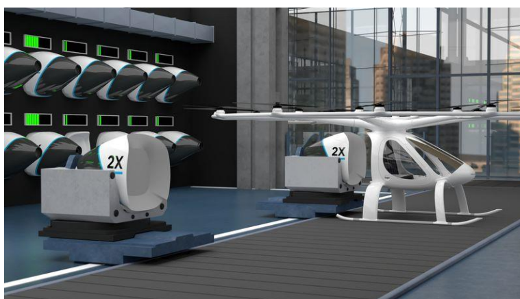
Figure 24. Battery pack swap concept by Volocopter [52]
